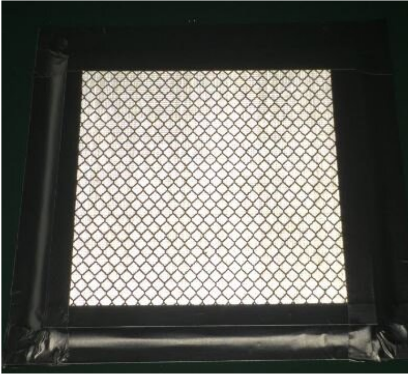
Surface appearance and structure of RR plate. Credit: Toyohashi University Of Technology.
