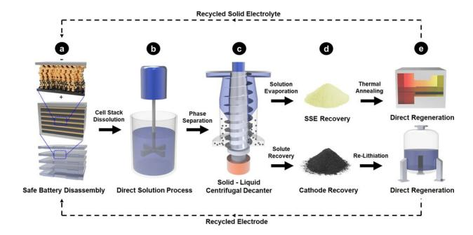
A proposed procedure for recycling solid-state battery packs directly and harvesting their materials for reuse. Credit: <u>Tan et al., 2020, CC BY</u>
