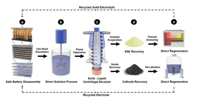
A proposed procedure for recycling solid-state battery packs directly and harvesting their materials for reuse. Credit: <u>Tan et al., 2020</u>, <u>CC BY</u>
