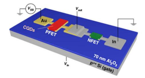
By depositing gold (Au) and Indium (In) contacts, researchers create two crucial types of quantum dot transistors on the same substrate, opening the door to a host of innovative electronics. Credit: Los Alamos National Laboratory
