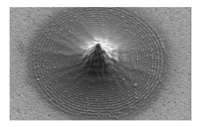
An on-chip carbonized electrode microstructure from a scanning electron microscope. Credit: ORNL, U.S. Dept. of Energy
