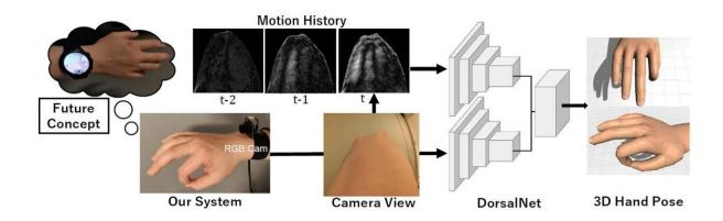
The system is the first of its kind to estimate 3-D hand poses using a camera focusing on the back of the hand. Credit: ACM, UIST
