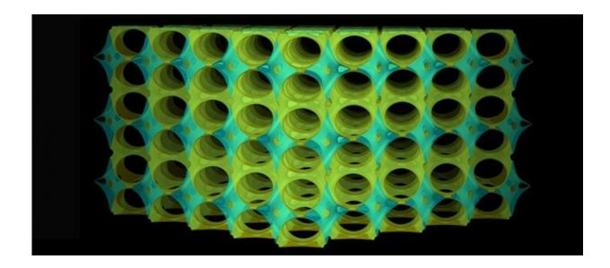
Three-dimensional surface of sodium ion diffusion in a hydroborate crystal. This new material forms a disordered yet highly symmetrical structure, allowing a mobility of sodium comparable to that of lithium in commercial battery. Credit: © UNIGE/Brighi
