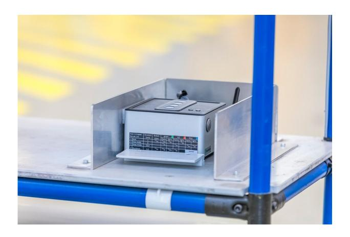
AirBOX in use: portable component monitoring on a material delivery unit or MDU. Credit: Fraunhofer IFF
