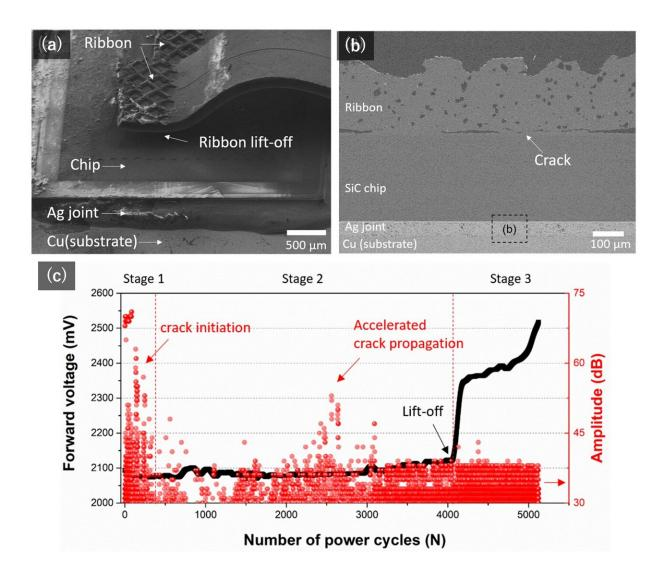
Figure 2. After eliminating background AE noise—including power on-off switching and ambient noise—via noise-filtering, AE signals were successfully collected for the SiC devices during a power cycling test. (a) Lift-off failure analysis results of failed discrete SiC-SBD devices after a power cycling test. (b) Cross section of one pre-failure Al ribbon where many cracks were observed at the interface. (c) AE single monitoring was compared with the traditional failure
