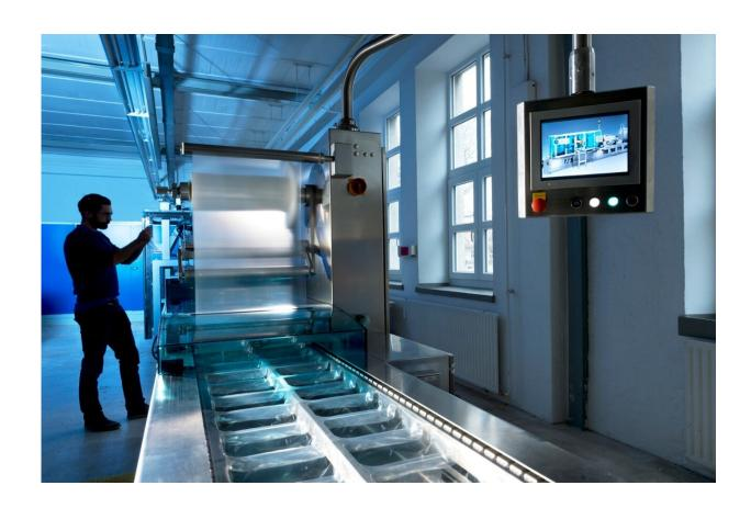
Demonstrator equipment at Fraunhofer IGCV – here a thermopackaging machine – shows how plant and associated machinery can be operated on an energy-adaptive basis. Credit: Fraunhofer IGCV/Bernd Müller
