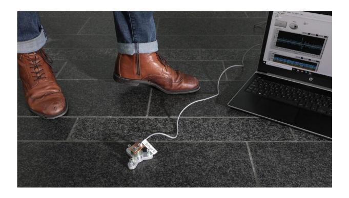
By installing sensors in a building's floor slabs, it's possible to measure the vibrations created by footsteps. Credit: EPFL, Alain Herzog
