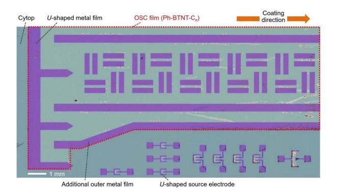
Optical microscopy image of organic thin film transistors etched in gold. Credit: © 2020 Kitahara et al.
