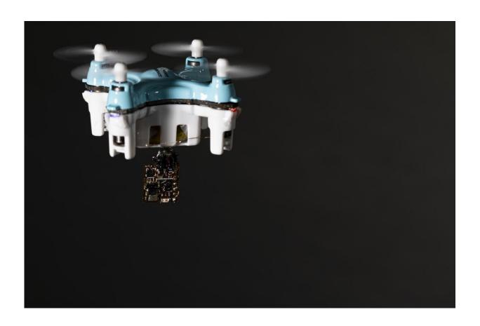
University of Washington researchers have created a 98 milligram sensor system—about one tenth the weight of a jellybean—that can be carried by a small drone. The drone shown here is a commercial quadcopter that was used in the experiments. Credit: Mark Stone/University of Washington
