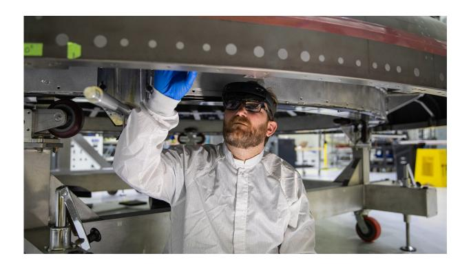
Eric Nolan, a technician working at the Kennedy Space Center, wears a HoloLens2 as he works on the heat shield for the crew module for NASA's Artemis II mission. Credit: NASA
