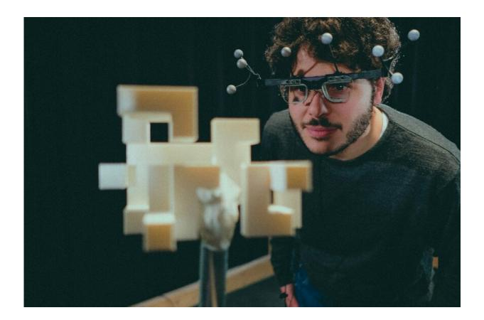
A subject performs a visual experiment using PESAO, equipped with the eyetracker, which has a motion tracking attachment installed. Credit: Solbach & Tsotsos.
