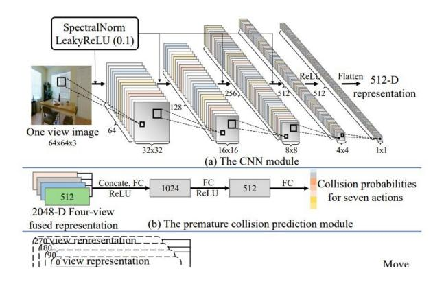
The architectures of the (a) CNN module, (b) premature collision prediction module, (c) target checking module developed by the researchers. Credit: Wu et al
