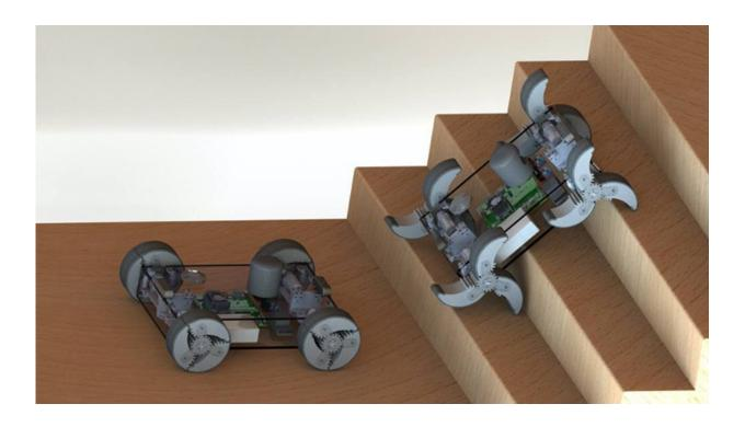
Concept illustration of the adaptable Wheel-and-Leg Transformable Robot currently being developed under a Defense Advanced Research Projects Agency contract. Credit: Kiju Lee
