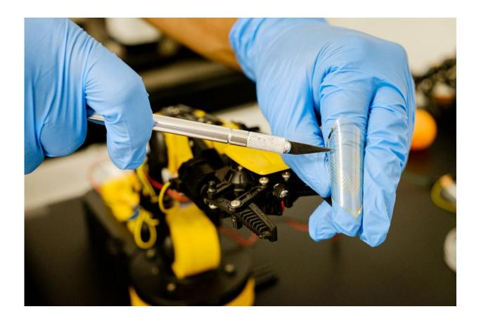
The system uses a type of self-healing ion gel material that enables the robot to restore its mechanical functions without human intervention when 'injured' with a cut from a sharp object. Credit: NTU Singapore
