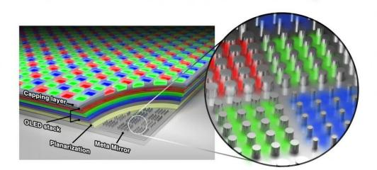
Illustration of the meta-OLED display and the underlying metaphotonic layer, which improves the overall brightness and color of the display while keeping it thin and energy efficient. Credit: Samsung Advanced Institute of Technology
