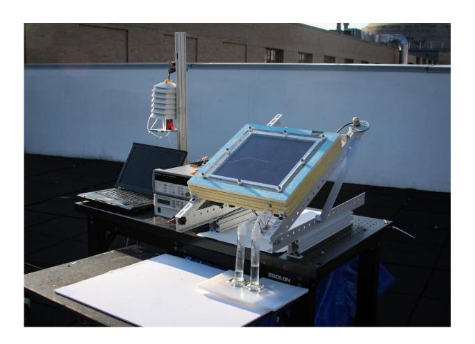
A prototype of the new two-stage water harvesting system (center right), was tested on an MIT rooftop. The device, which was connected to a laptop for data collection and was mounted at an angle to face the sun, has a black solar collecting plate at the top, and the water it produced flowed into two tubes at bottom.Credit: Alina LaPotin
