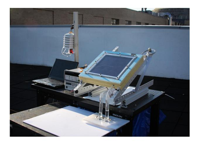
A prototype of the new two-stage water harvesting system (center right), was tested on an MIT rooftop. The device, which was connected to a laptop for data collection and was mounted at an angle to face the sun, has a black solar collecting plate at the top, and the water it produced flowed into two tubes at bottom.Credit: Alina LaPotin
