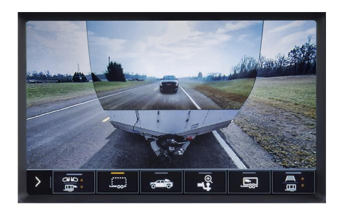
This image provided by General Motors, shows the display of a 2020 GMC Sierra HD feature called Transparent Trailer, one of the few pickup trucks that provides an image of the road behind a trailer. This optional feature uses augmented reality to project an image of the road on the front of a trailer, giving the illusion of a transparent trailer. (General Motors via AP)
