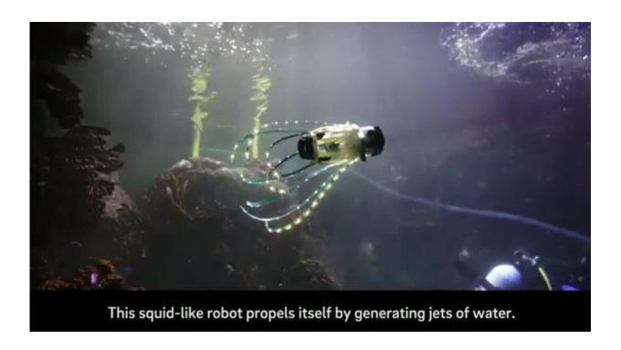
Engineers at the University of California San Diego have built a squidlike robot that can swim untethered, propelling itself by generating jets of water. The robot carries its own power source inside its body. It can also carry a sensor, such as a camera, for underwater exploration.
