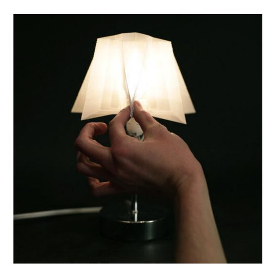
In this deformation-sensing lamp, the solid supports, textile lampshade, and sensing conductive pads are created as a single print. Credit: Jack Forman
