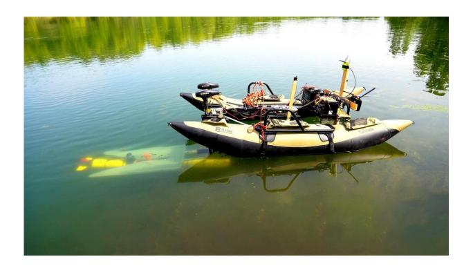
A yellow underwater robot (left) finds its way to a mobile docking station to recharge and upload data before continuing a task. Credit: Purdue University photo/Jared Pike
