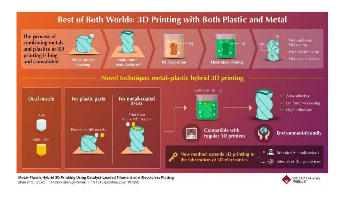
An approach that extends the use of 3-D printers to 3-D electronics for future robotics and Internet-of-Things applications Credit: Waseda University
