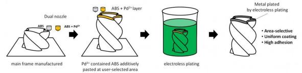
Overview of the conventional and the proposed method for the metallization of a 3D-printed plastic structure. Unlike the conventional technique, the proposed dual-nozzle approach produces 3D objects with a uniform and strongly adhered metallic coating in desired areas only. Credit: Shinjiro Umezu
