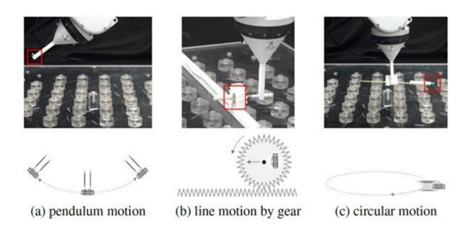
When the motion contains occasional dead-angle data, the result is wrong, but it can be reconstructed with filters. The performance of the proposed structureaware temporal bilateral filter surpasses any other conventional filters because it leverages raw measurement of the sensors. Credit: Tohoku University
