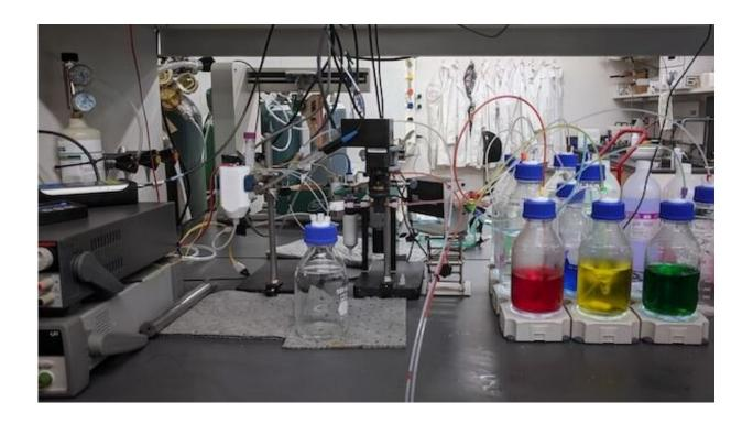
"Otto" is a robotic platform integrated with machine learning to optimize electrolytes for batteries. Credit: College of Engineering, Carnegie Mellon University
