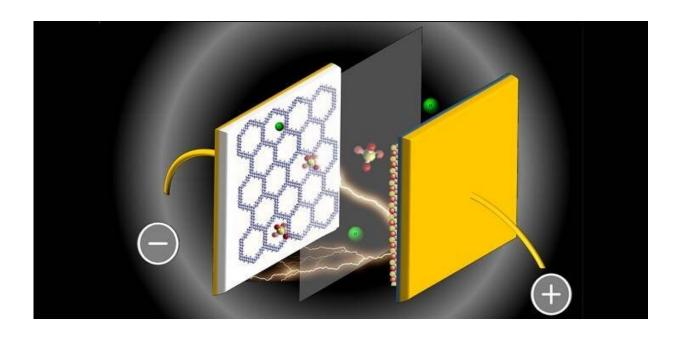
Schematic depiction of the asymmetric supercapacitor with the porous COF as the negative electrode shown on the left. Credit: KAUST, Osama Shekhah
