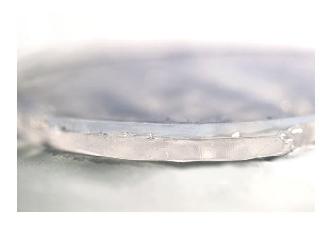
MIT researchers have developed a two-layer passive cooling system, made of hydrogel and aerogel, that can keep foods and pharmaceuticals cool for days without the need for electricity. In this photo showing a close-up of the two-layer material, the upper layer consists of aerogel and the bottom layer of hydrogel. Credit: Jeffrey Grossman, et. al
