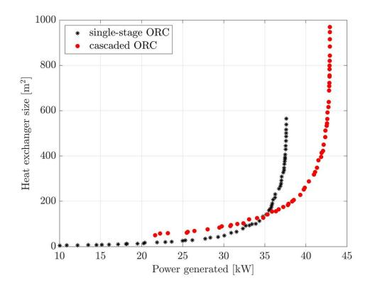
The red and black markers correspond to the Pareto fronts generated for the two different systems, leading to two inferences: If quite large heat exchangers (in this specific case, greater than around 200m2), were affordable, then for that amount of area, it is possible to generate more power with a cascaded system than a single-stage system. Credit: Dr. Martin White, City, University of London
