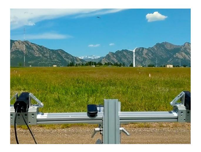
ThermalTracker-3D tracks an unmanned aerial system (visible top, center) during testing at the NREL Flatirons Campus. Credit: Shari Matzner, PNNL
