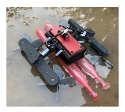
A new high-speed amphibious robot inspired by the movements of cockroaches and lizards, developed by Ben-Gurion University of the Negev (BGU) researchers, swims and runs on top of water at high speeds and crawls on difficult terrain. Credit: credit: Ben-Gurion University
