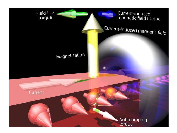
Field-like torque tries to align the magnetization with the plane of the material, but to work as a memory device the magnetization needs to be perpendicular to this. Credit: 2020 Ohya et al.
