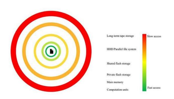
Orchestrating the movement of data between more remote storage layers and main memory can speed up simulations by 2.5 times. Credit: KAUST
