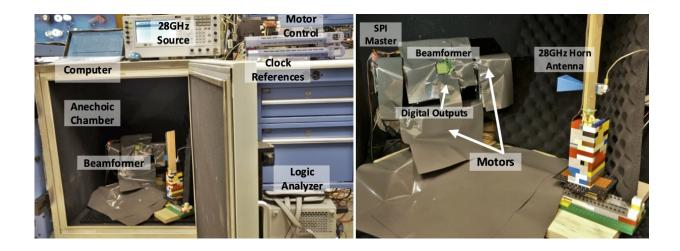
Test setup built by the students includes a mini anechoic chamber, and a mechanical device to move the beamformer in order to test its accuracy. Credit: University of Michigan
