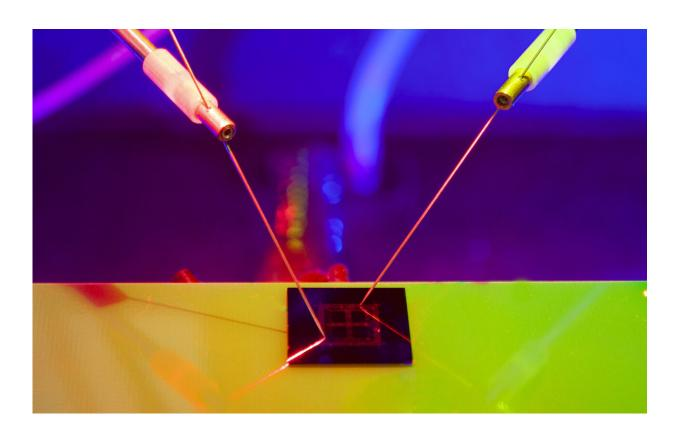
The light-powered AI chip - prototype technology that brings together imaging, processing, machine learning and memory. Credit: RMIT University
