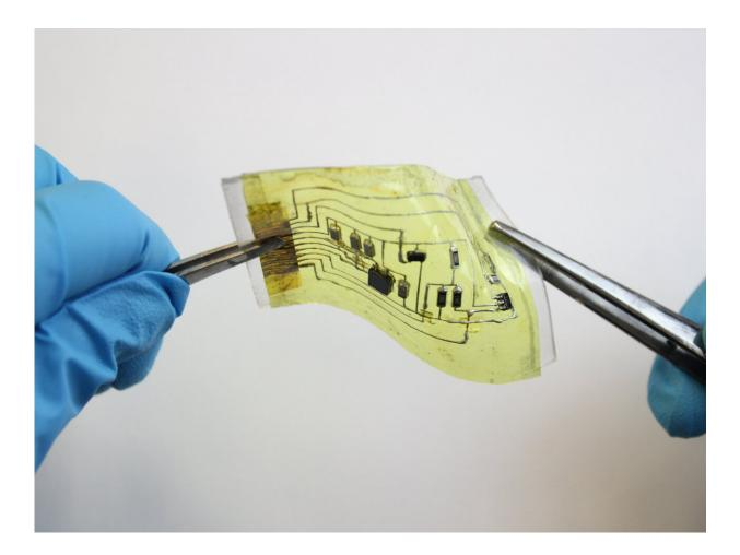
A new "electronic skin" device can stretch by 60% in any direction without losing any functionality. Credit: Chuanqian Shi
