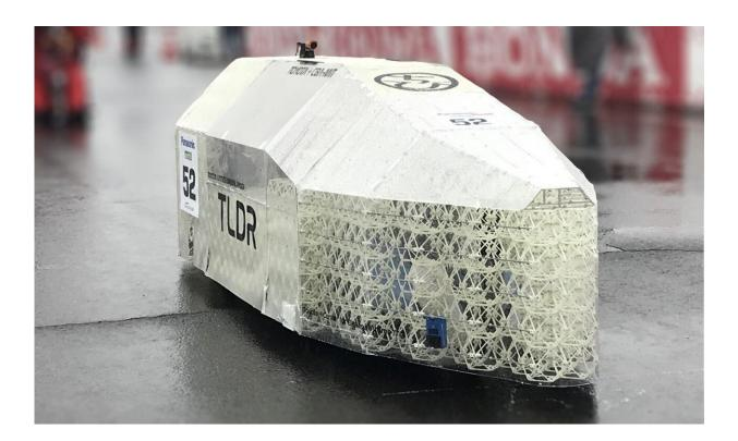
Army and MIT's way of linking metamaterials makes building a supermileage vehicles, like this one from collaborators Toyota Automotive Society, possible. Supermileage vehicles aim to get the most mileage out of a single tank of highoctane gasoline. Credit: (Kohshi Katoh, Toyota Automotive Society)
