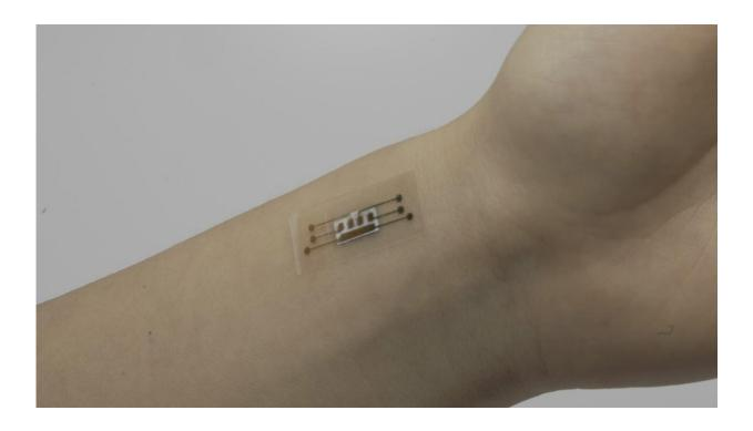
Flexible TRACE sensor patches can be placed on the skin to measure blood flow in superficial arteries. Credit: National University of Singapore
