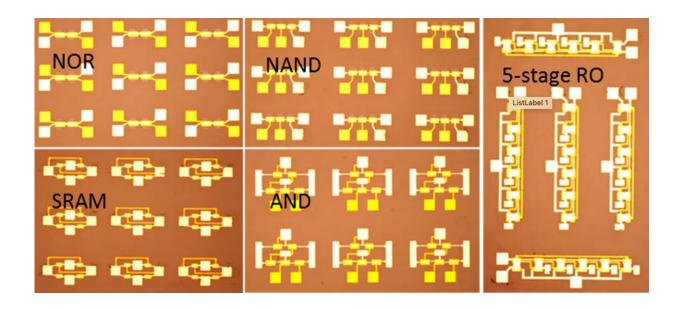
Photographs of different MoS2 integrated devices including inverters, NOR gates, NAND gates, SRAMs, AND gates, and 5-stage ring oscillators. Credit: Li et al.
