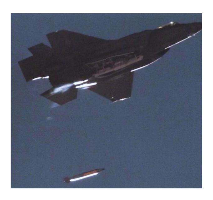
An F-35A Lightning II opens its bomb bay doors and drops a mock B61-12 at Sandia National Laboratories' Tonopah Test Range. Credit: Sandia National
