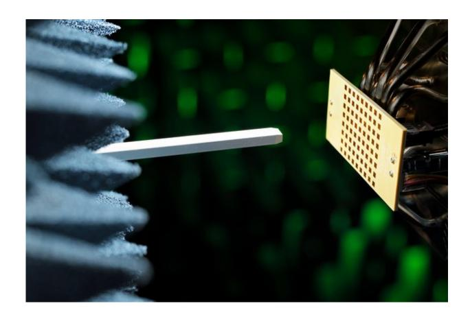
The front side of the developed module in a measurement setup, including its 72 antenna elements. Credit: Eindhoven University of Technology
