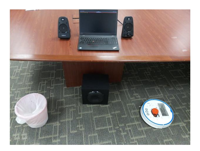
Researchers repurposed the laser-based navigation system on a vacuum robot (right) to pick up sound vibrations and capture human speech bouncing off objects like a trash can placed near a computer speaker on the floor. Credit: Sriram Sami
