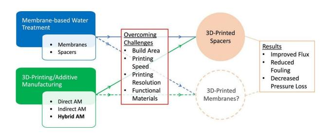
Overview of the relationship between 3D printing and membrane-based water treatment industry. Credit: SUTD
