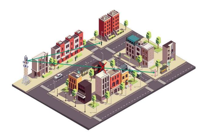
A communication scenario in an urban area before the deployment of RISs that shows how one user does not have a line of sight with the base station. Credit: KAUST; Mustafa Kishk & Maha M. Kamal
