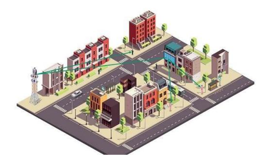
Reconfigurable intelligent surfaces (RISs) on buildings could significantly improve communication network coverage. The RIS system could eliminate blind spots by redirecting signals that would otherwise be blocked by buildings. Credit: KAUST, Mustafa Kishk & Maha M. Kamal
