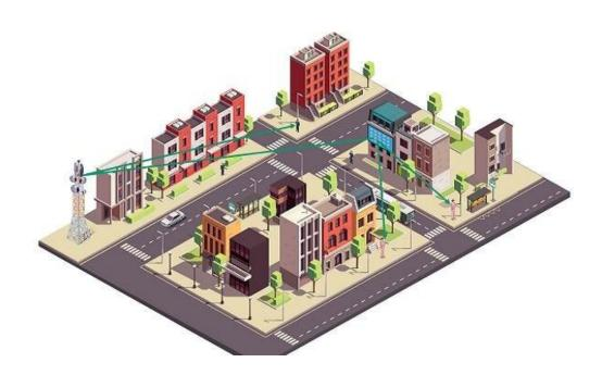
Reconfigurable intelligent surfaces (RISs) on buildings could significantly improve communication network coverage. The RIS system could eliminate blind spots by redirecting signals that would otherwise be blocked by buildings. Credit: KAUST, Mustafa Kishk & Maha M. Kamal
