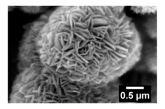
A scanning electron microscope image of lithium titanate (lithium, titanium, oxygen) "nanoflowers." Credit: Brookhaven National Laboratory
