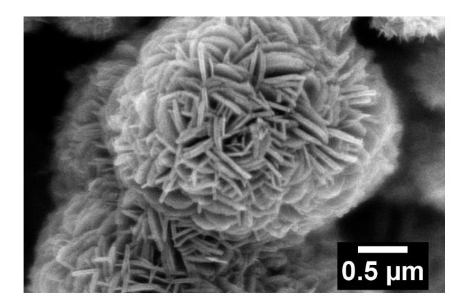
A scanning electron microscope image of lithium titanate (lithium, titanium, oxygen) "nanoflowers." Credit: Brookhaven National Laboratory
