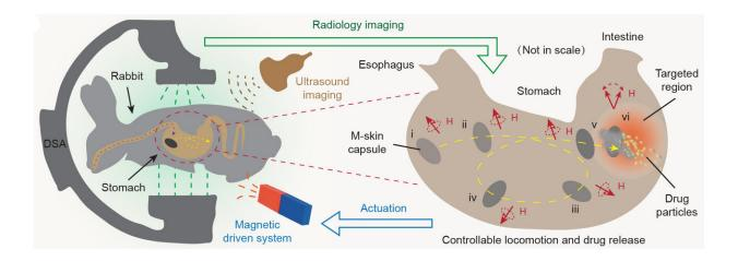
Schematic of the drug delivery in rabbit stomach. The magnetic field is applied for robot actuation, radiology imaging is adopted for locomotion evaluation, and ultrasound imaging is adopted for drug release evaluation. Credit: Yang et al., Sci. Robot. 5, eabc8191 (2020)
