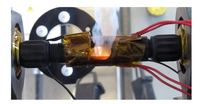
If there were a spark, a special polymer, developed by Sandia National Laboratories, within the in-line connectors would melt and a spring would extend inside the connector to facilitate a larger spark gap and stop the flames, as shown in this photo. Credit: Kenny Armijo
