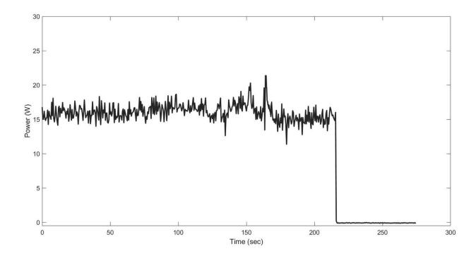
This image shows an example of an in-line connector test conducted at Sandia National Laboratories at the moment of an arc-fault and sudden self-extinguishment. The graph depicts a sudden voltage drop that occurred in less than a second when the in-line connector extinguished a spark. Credit: Kenny Armijo
