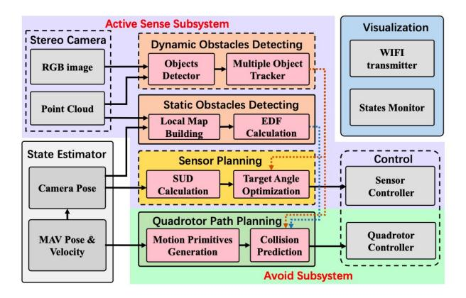
An overview of the active sense and avoid (ASAA) system developed by the researchers. Credit: Chen et al.
