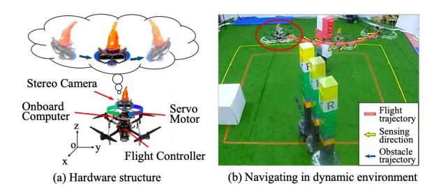
The flying robot used by the researchers operating in a dynamic environment. (a) the system's hardware structure. (b) a scenario in which the flying robot maneuvers through the gap between a dynamic and a static obstacle. Credit: Chen et al.
