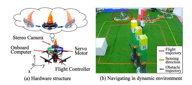
The flying robot used by the researchers operating in a dynamic environment. (a) the system's hardware structure. (b) a scenario in which the flying robot maneuvers through the gap between a dynamic and a static obstacle. Credit: Chen et al.
