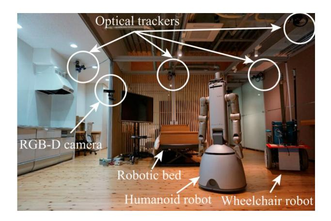
The researchers' experimental setup. An optical tracking system tracks robots and objects inside the room, while RGB-D cameras primarily track human motion. Credit: Egashira et al.
