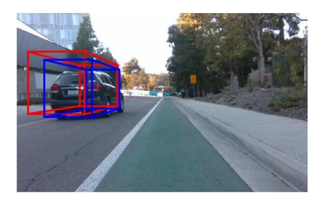
Multi-radar system predicting the dimensions of cars in live traffic. Red boxes are the predictions, blue boxes are the ground truth measurements. Credit: Kshitiz Bansal
