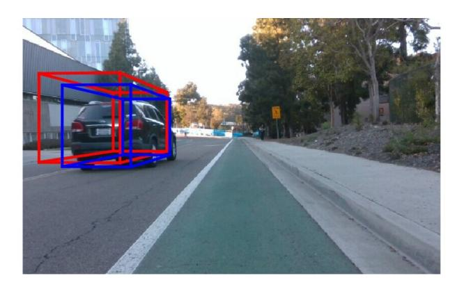
Multi-radar system predicting the dimensions of cars in live traffic. Red boxes are the predictions, blue boxes are the ground truth measurements. Credit: Kshitiz Bansal
